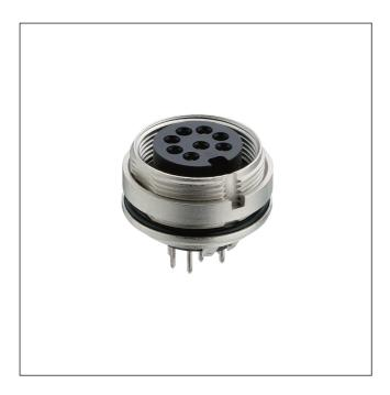
SWUM<sup>™</sup> chassis socket acc. to IEC 61076-2-106 and AISG specification, IP 68/67, with threaded joint, for printed circuit boards, manual soldering, for back side mounting
